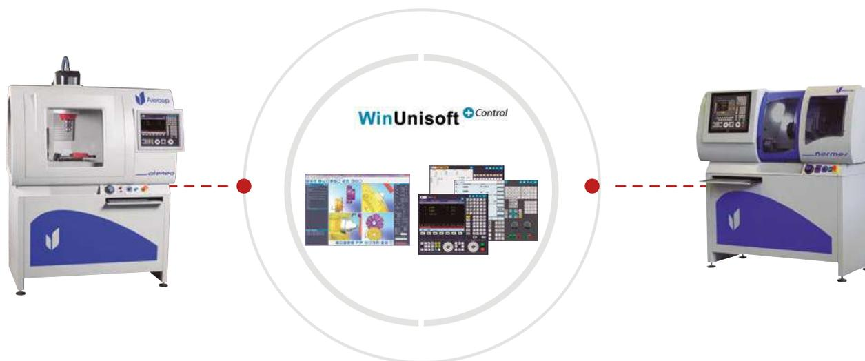
Using the features of a local network the teacher can share projects created in the machine with WinUnisoft<sup>+</sup>. The students can use the simulation of WinUnisoft<sup>+</sup> on their PCs to work with the same machine/tools/workpiece configuration and create their own programs.
