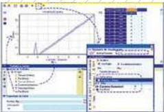
In each test a set of signals are collected a signal that is stored in the results. With DIANA signals can be viewed, compared, operations can be carried out among them and filters can even be applied.
