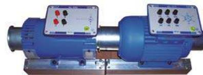
Three-phase asynchronous motor **AL-1106**
